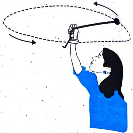
Fig. 5.4 Force is necessary for changing the direction of momentum, even if its magnitude is constant. We can feel this while rotating a stone in a horizontal circle with uniform speed by means of a string.
