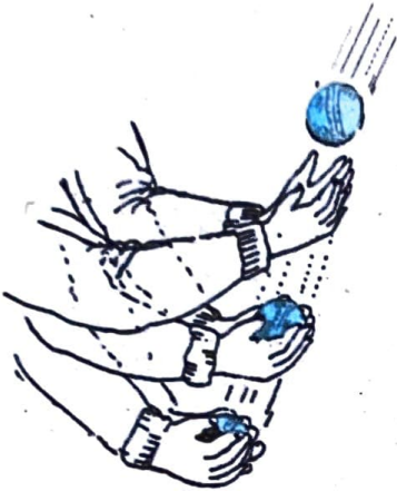
Fig. 5.3 Force not only depends on the change in momentum but also on how fast the change is brought about. A seasoned cricketer draws in his hands during a catch, allowing greater time for the ball to stop and hence requires a smaller force.
