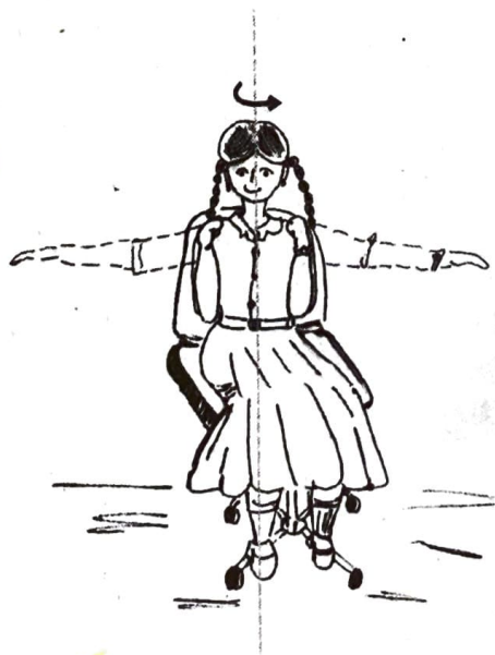
Fig 7.36 (a) A demonstration of conservation of angular momentum. A girl sits on a swivel chair and stretches her arms/ brings her arms closer to the body.
