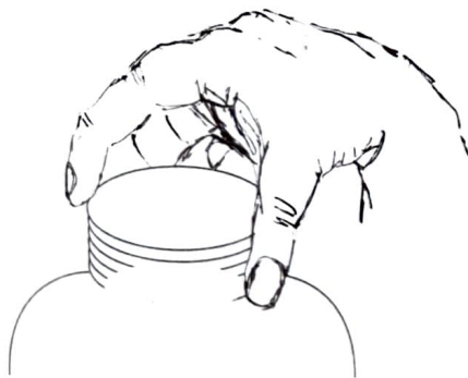
Fig. 7.21(a) Our fingers apply a couple to turn the lid.
